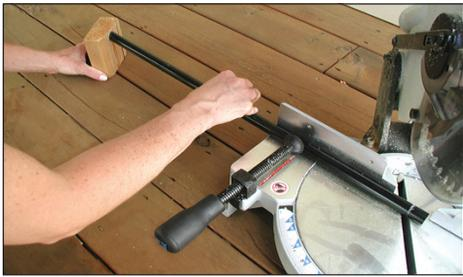
**Step 4:** Flip the baluster and clamp tightly. The second cut is parallel to the first cut. Place a square block against the first cut end. Spin the baluster until the full rim is in contact with the block. Tighten with a clamp and trim. The block must be square to ensure an accurate parallel cut.
