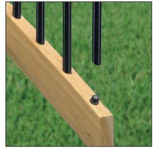
**Step 7:** Slide the trimmed balusters over each FastBall baluster connector on the bottom rail. Use a rubber mallet to tap the balusters onto the connectors if needed. Install the top rail, fitting balusters on each FastBall connector as you work across. Gently tap the top rail with a rubber mallet to eliminate any gaps. Secure handrail to post according to local building codes.
