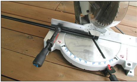
**Step 3:** Clamp the baluster to the guard and trim using a carbide tip blade. Use a fixture to consistently cut each baluster.
