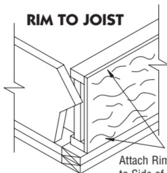
Attach Rim Board to Side of OPEN JOIST With 8d Nails at 4" o.c. Into Top and Bottom Chords
