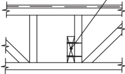
Framer is Advised to Install and Nail All Strongbacks Before Installation of the Sub Floor.
