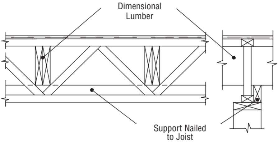
NOTE: Cantilevered Dimensional Lumber must be engineered for load and deflection per applicable code.
