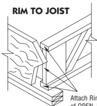
Attach Rim Board to End of OPEN JOIST With (1) 8d Nail at Each Flange and (1) 8d Nail Centered at End Block
