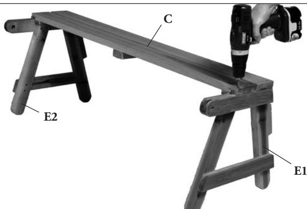
**STEP 1** Attach the shorter seat (**C**) to the two table legs (**E1** & **E2**) using eight 3.5 x 35mm wood screws through the pre-drilled holes. Turn seat upside down.
