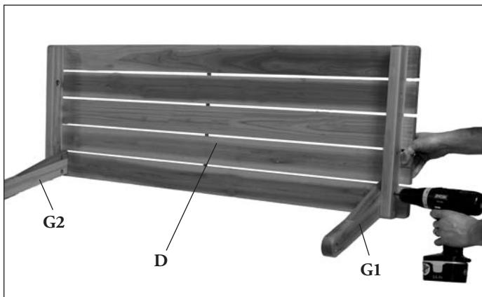
**STEP 3** Place the tabletop hinges (**G1 & G2**) to the inside of the tabletop cross members. Attach tabletop hinges to the tabletop (**D**) using four 6 x 25mm machine screws.
