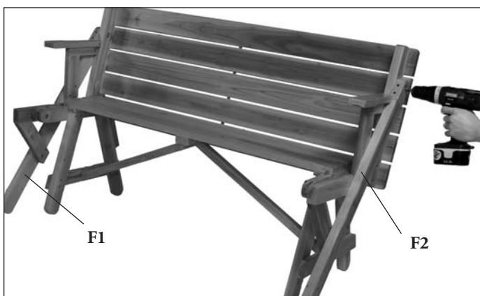
**STEP 5** Place the table legs with armrests (**F1 & F2**) to the outside of the opposite end of the tabletop cross members and attach using two 6 x 25mm machine screws.
