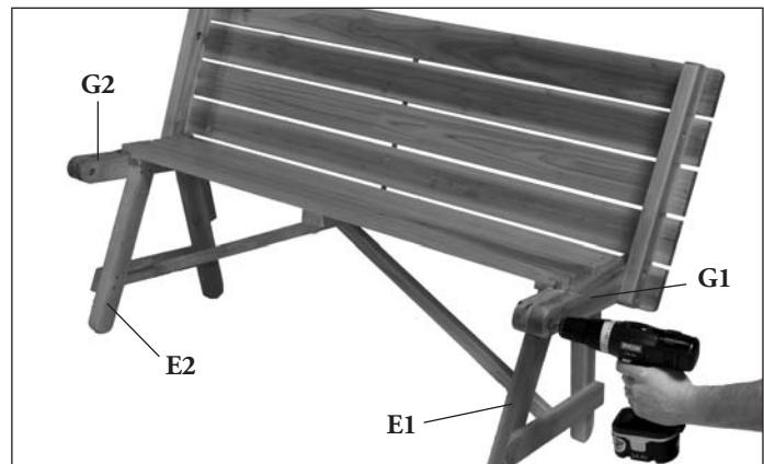
**STEP 4** The opposite ends of the tabletop hinges fit to the outside of the table legs. Attach tabletop hinges (**G1 & G2**) to the table legs (**E1 & E2**) using two 6 x 25mm machine screws.
