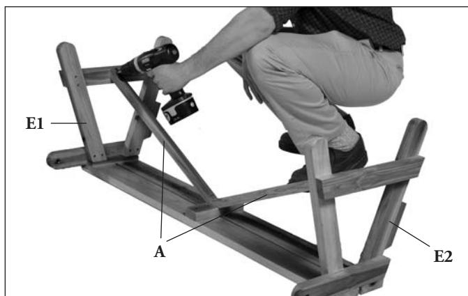
**STEP 2** Make sure the legs are perpendicular to the seat and attach diagonal braces (**A**) using four 3.5 x 25mm screws. The double-beveled ends of the diagonal braces will meet at the center of the seat.
