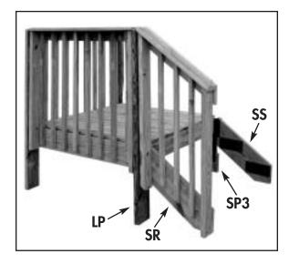
7. Slide stair rail section (SR) onto the line post connectors (LP). This is best achieved by lining up the longer bottom connectors prior to sliding the connectors together. Slide the stair stringer onto the sub post (SP3). Secure by tapping with a rubber mallet.
