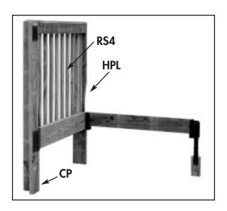
2. Slide a 4' handrail section (RS4) onto the corner post (CP),making sure the corner post connectors on the adjacent side of the post face toward the deck. This is best achieved by lining up the longer bottom connectors prior to sliding the connectors together. Slide the opposite end of the rail section (RS4) onto the house post (HP). Secure to posts by tapping each side of rail section with a rubber mallet.
