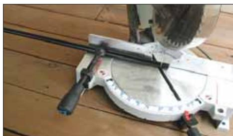
**Step 3:** Clamp the baluster to the guard and trim using a carbide tip blade. Use a fixture to consistently cut each baluster.
